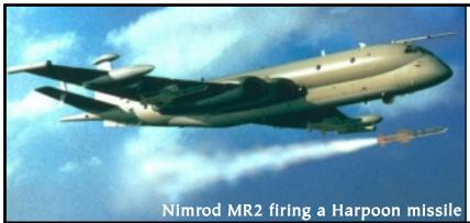
Canada's Lt.Col. Jason Major flew a British Nimrod MR2 during the Iraq war, in 2003. These spy planes are armed with Sidewinder air-to-air missiles, Stingray anti-sub torpedoes, and Harpoon anti-ship missiles. They were also fitted with L3 Wescam's MX-15 target-finding sensor turret made in Canada.
