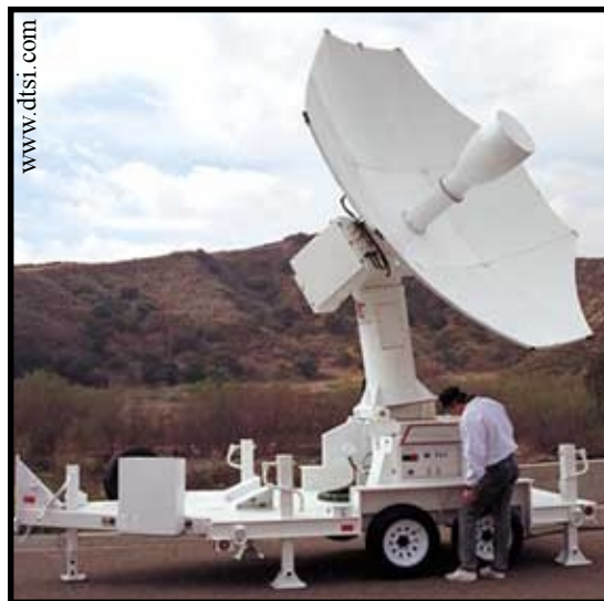
"The Eagle Vision system, deployed to the United Arab Emirates in support of Operation Iraqi Freedom, is an in-theater direct downlink of commercial satellite imagery."
